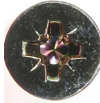
PZ Before Installation
